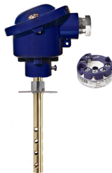
9409601 Type 9440 for ventilation with transmitter T15 with output signal 4-20 mA Perforated insertion tube of brass L-110x10 mm
